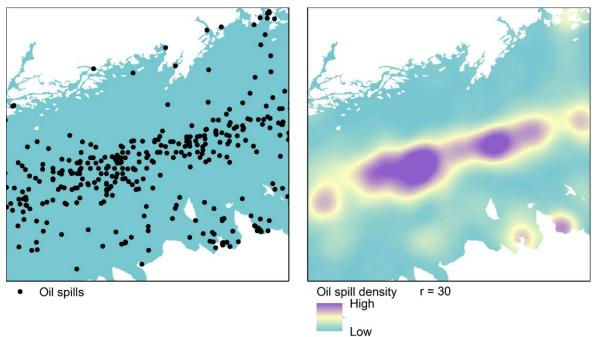
Figure 8. A heat map visualisation of marine oil spill point data (with Kernel density search radius r = 30). The original point data has a large number of overlapping observations, making it challenging to visualise.
